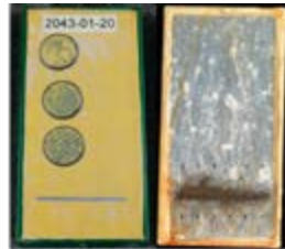
Figure 2. Initial trials after CX testing To the left: silicate topcoat. To the right reference
